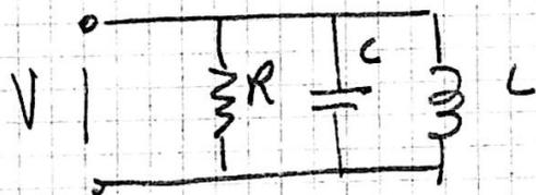
$$\frac{\omega_0 \frac{1}{2} C V_m^2}{\left( \frac{V_m}{\sqrt{2}} \right)^2 \frac{1}{R}} = \omega_0 C R = \frac{R}{\omega_0 L}$$
